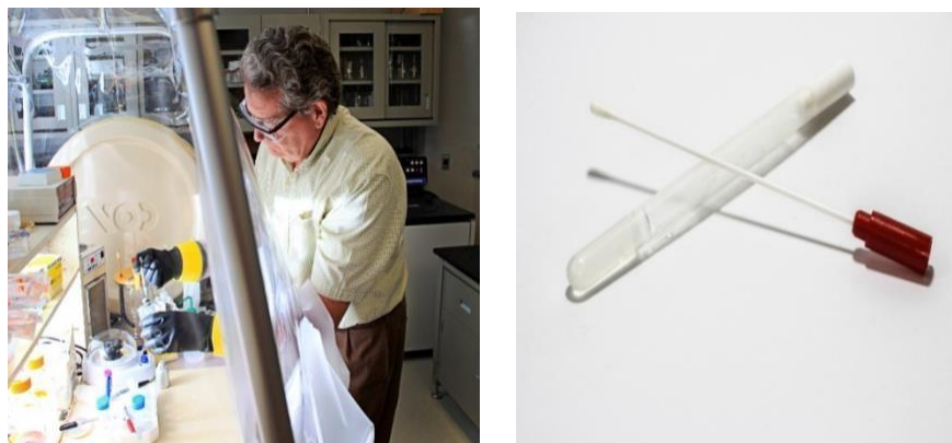
Figure 6.1: Microbiologists use anaerobic glove boxes to work with bacteria that require oxygen-free conditions (left); a culture transport system (right).
